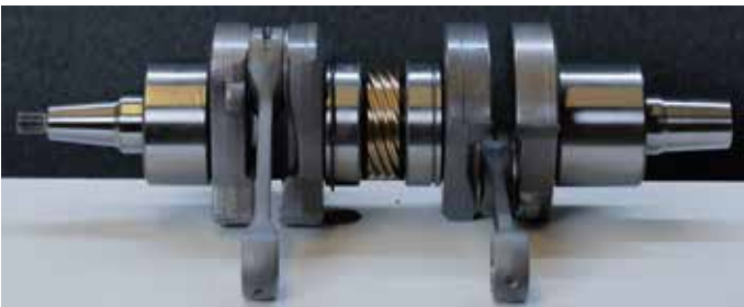
61-800KC 2205648, 2207761, 2208212 Note: Machined web, light weight
